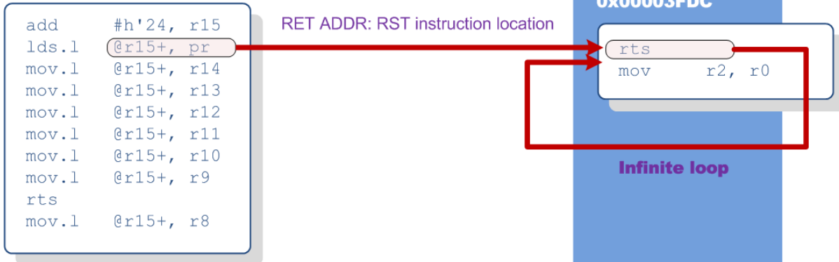
Fig. 19 Illustration of an Infinite loop through the rts instruction.
