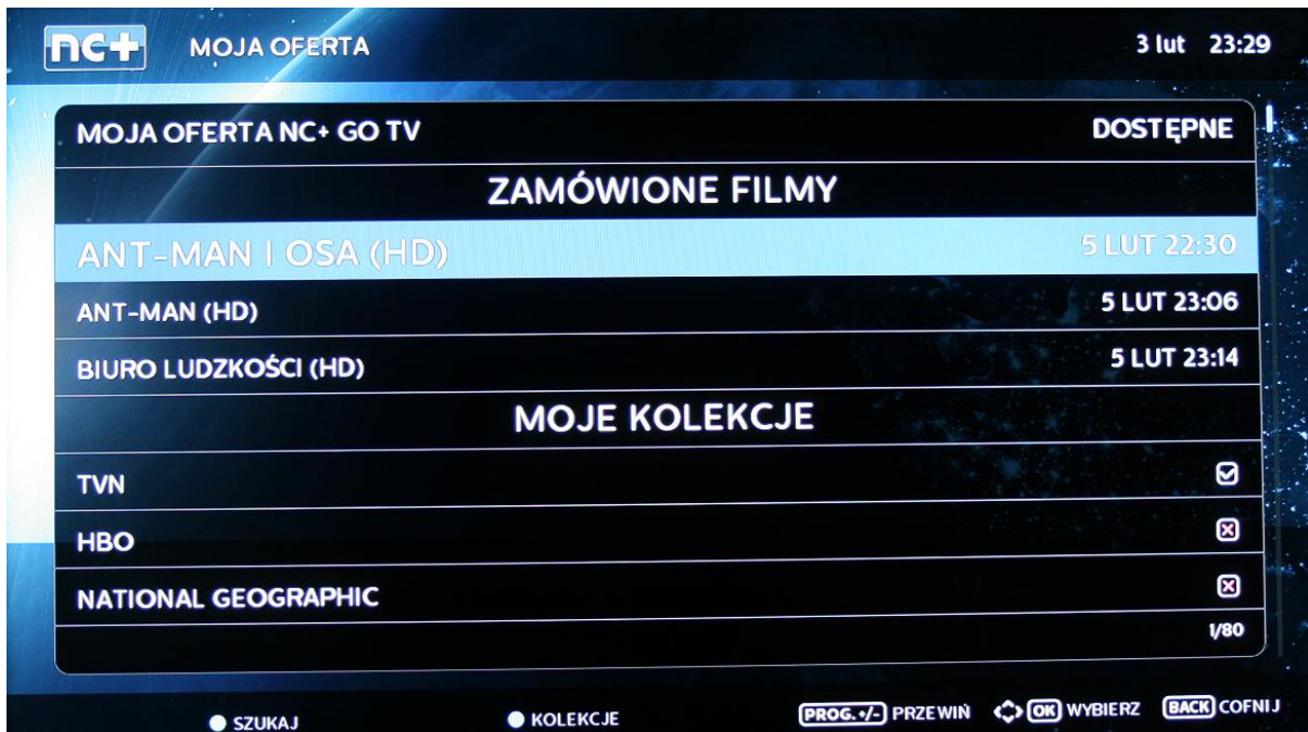
Fig. 36 STB screen indicating successful VOD orders conducted through JSON API and arbitrary price input.
