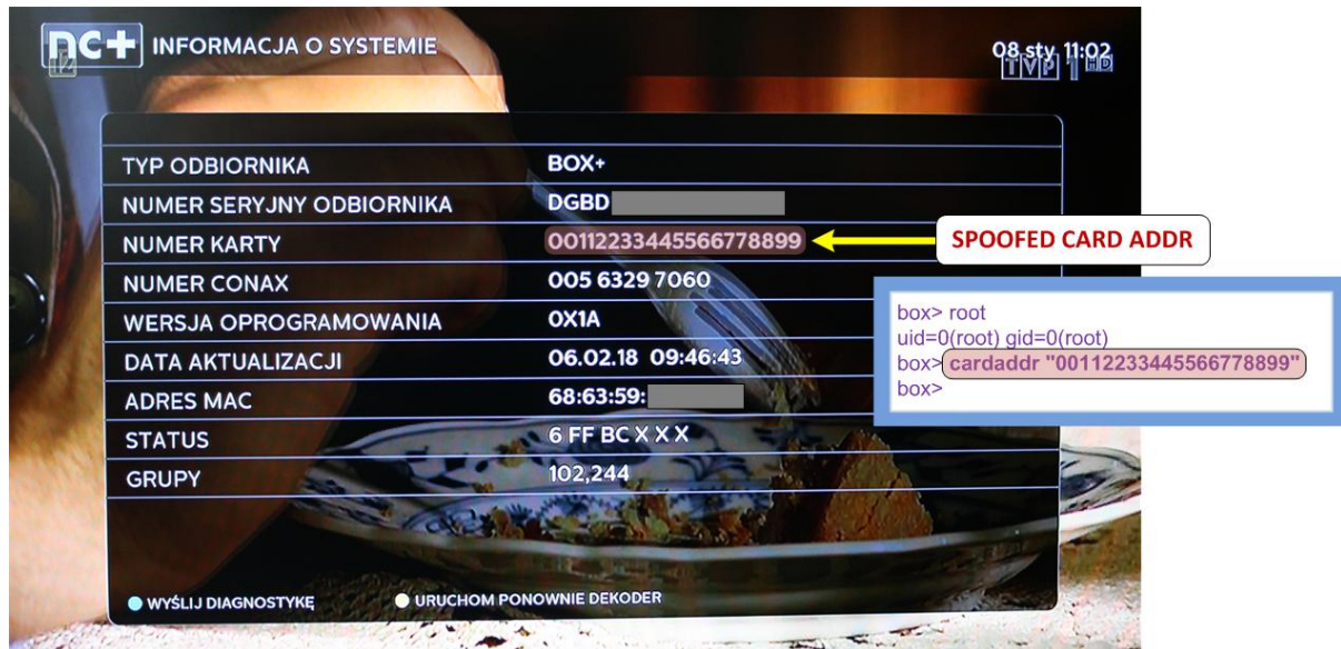
Fig. 26 Spoofing STBs smart card address.
